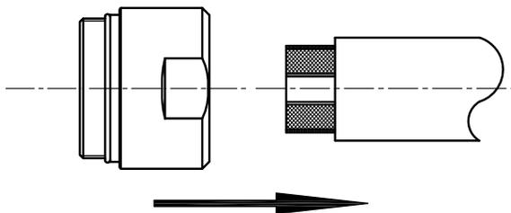
3. Spread out Outer Conductor as shown
