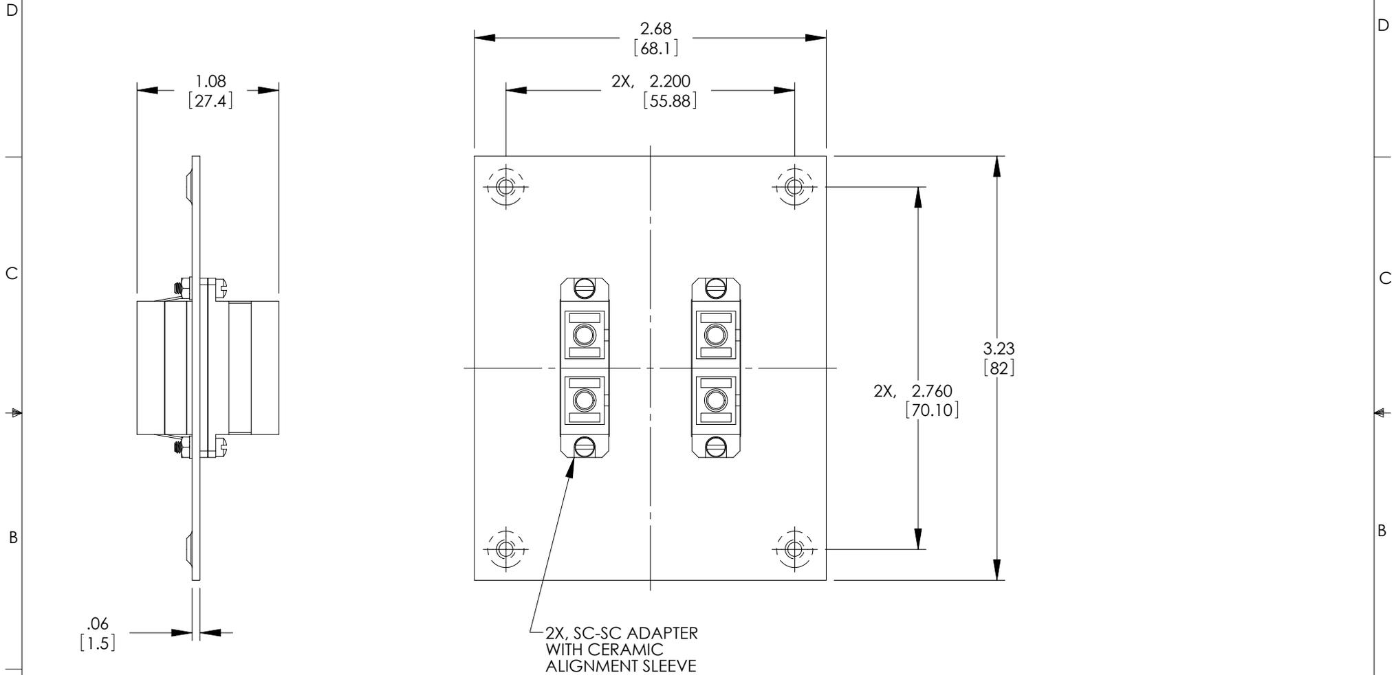
2X, SC-SC ADAPTER WITH CERAMIC ALIGNMENT SLEEVE
