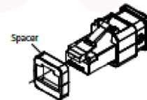
Step 3: After spacer installation, glide the bracket from the back and fasten using M2.6 x 5.0mm screw provided
